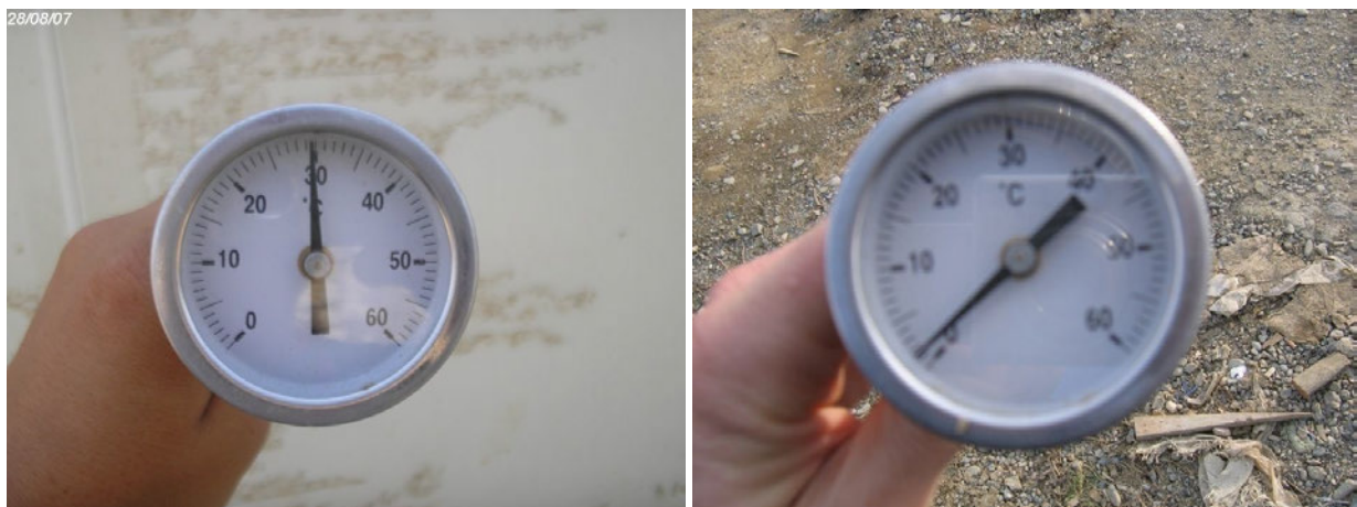
Picture 34: Thermometers on site measuring unacceptable temperatures. (Photo: ADA Project Archive)
