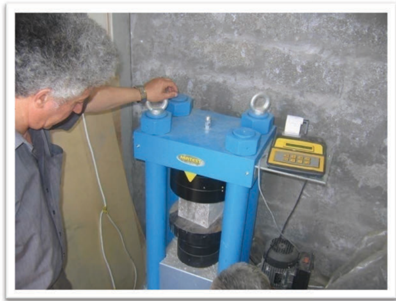
Picture 33. Cubes are tested in hydraulic press. (Photo: ADA Project Archive)
