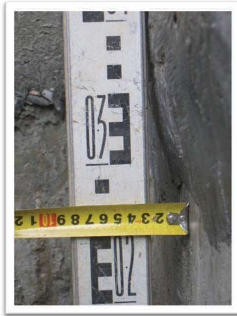
Picture 25: The Ruling Ruler; Measuring a Dent. (Photo: ADA Project Archive)
